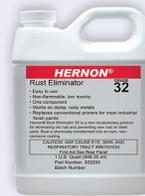
Chemically changes rust to a tough protective coating and primes the surface for painting. A single treatment can last for years. Wire brush and apply two or three coats. No need to sandblast or prime surfaces. Coating withstands constant temperatures to 200°F, and intermittent exposure to 250°F. Makes easy work of routine maintenance on machinery.
